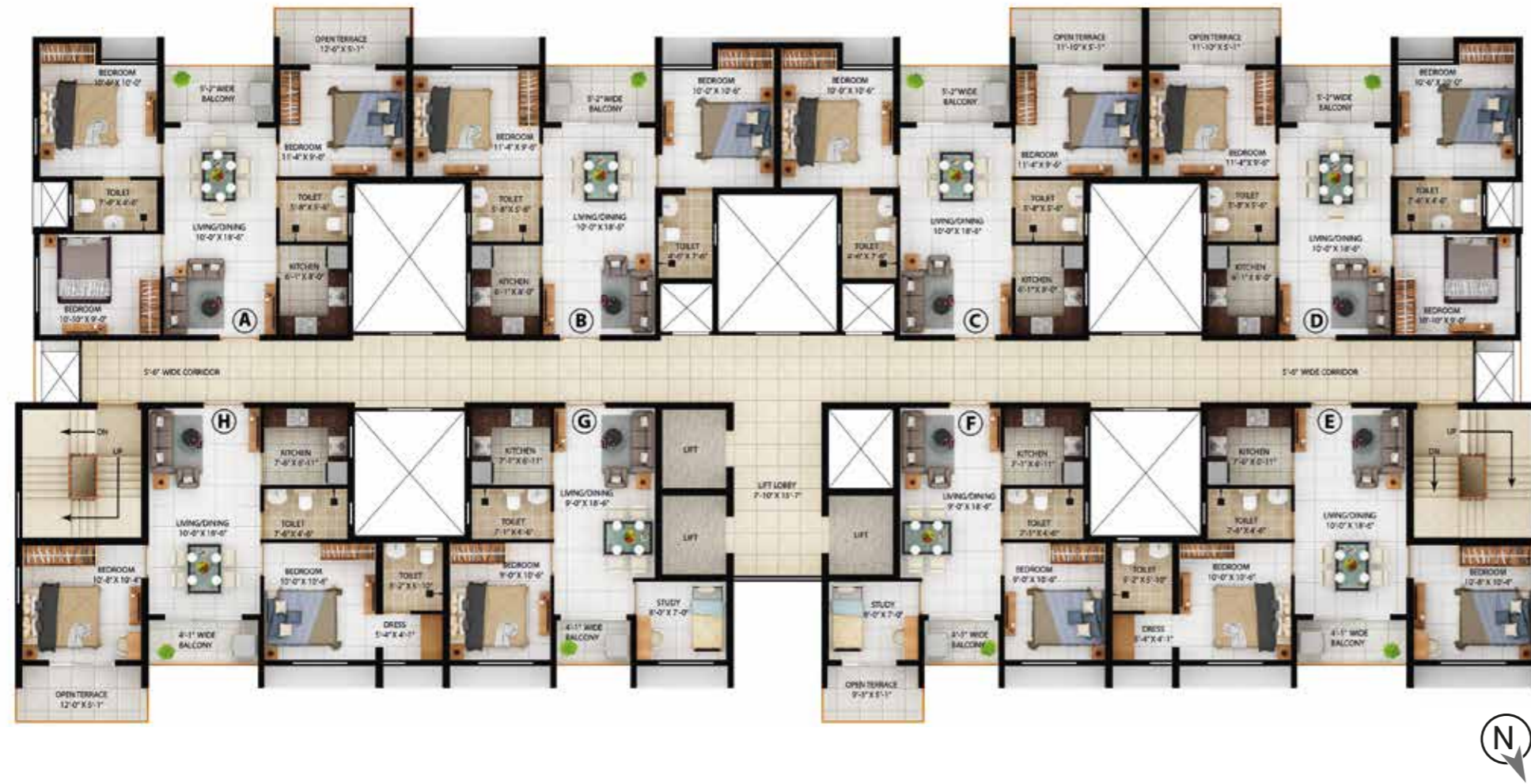
RIA (BLOCK 3B) | Typical floor plan (2nd, 5th, 8th & 11th Floor Plan)
